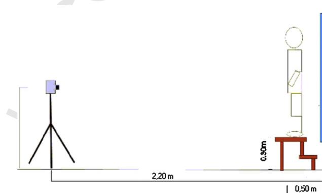
Figure 1 Schematic draw of the photographic method.
